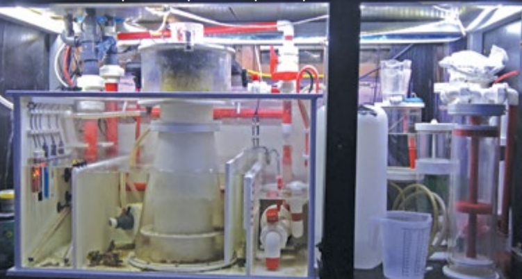
Vertex I-Supra C+ sump with an Alpha 250 protein skimmer
