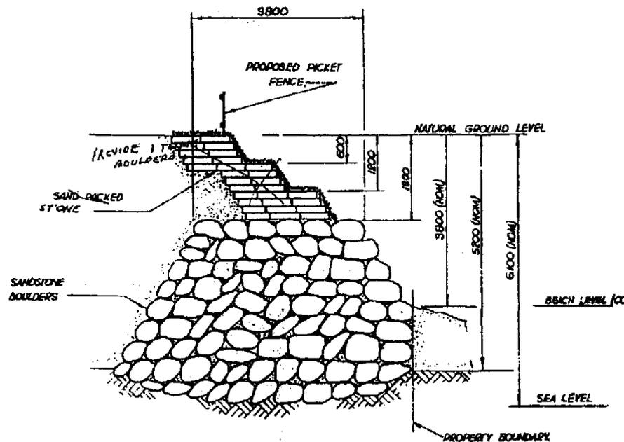
**Figure A25: 1978 design drawing for 23 Surfview Road revetment from WRL (1999), note upper section as drawn has hand written notes showing this was deleted and replaced by boulders**
