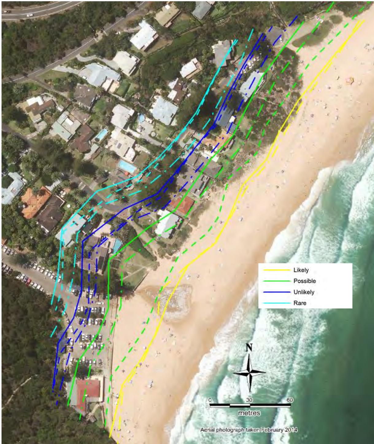
**Figure D9: 95% (dash dot line), 50% (solid line) and 5% (dashed line) exceedance recession scenario likelihood lines at Bilgola Beach for Type 2 procedure for 60 year design life (at 2075)**
