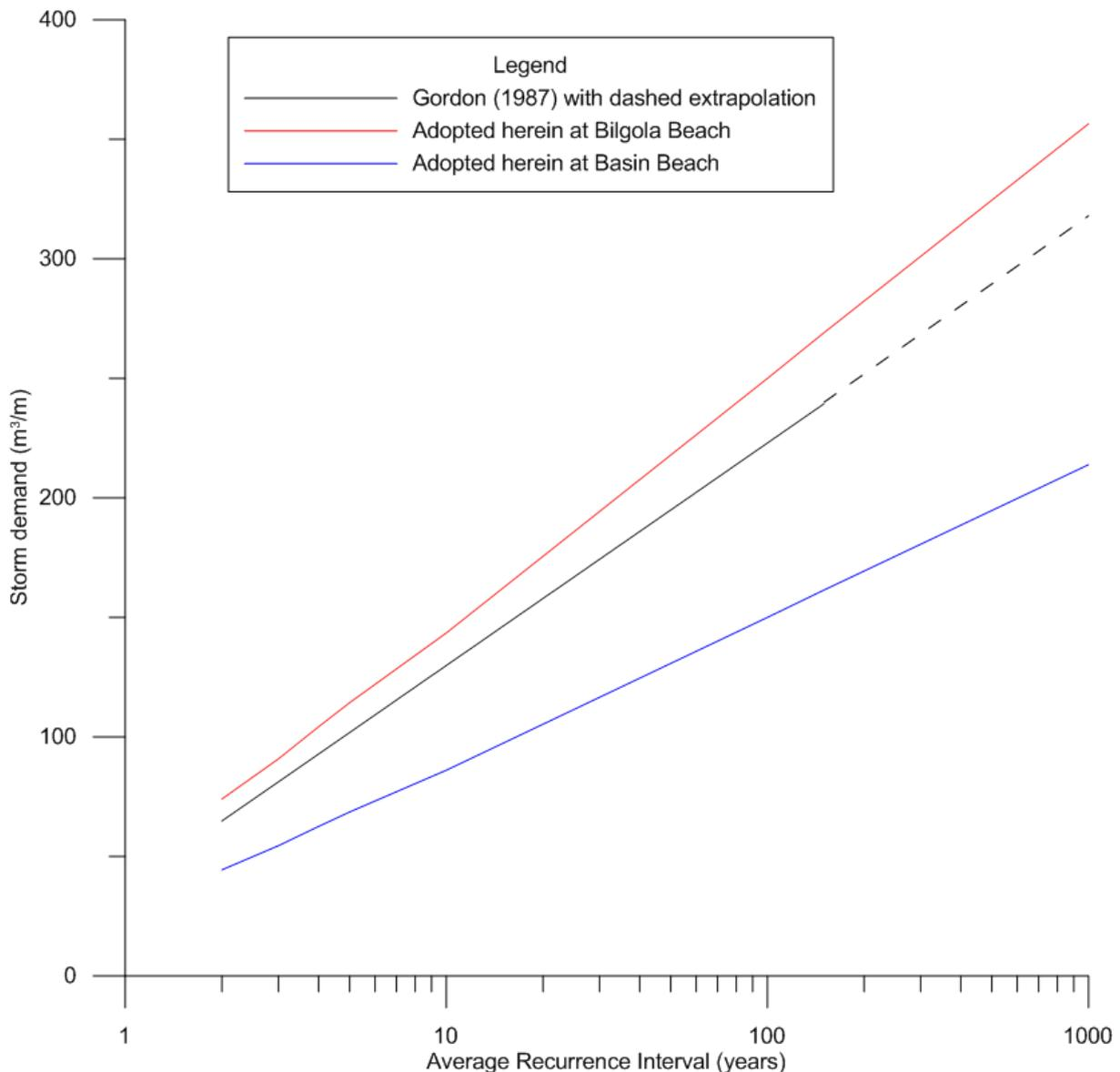
**Figure D1: Relationship between storm demand and ARI as developed by Gordon (1987) for “high demand” (rip head) areas, along with adopted values for investigation herein**
