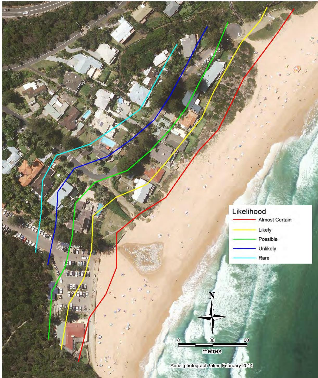
**Figure D7: Likelihood lines at Bilgola Beach for Type 1 procedure (no recession included) for 60 year design life (to 2075)**
