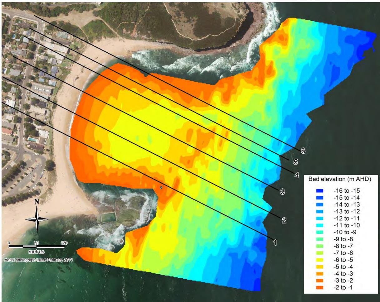
**Figure D4: Bathymetric contours (relative to AHD) at Basin Beach from May 2014 OEH survey (1m contour interval)**
