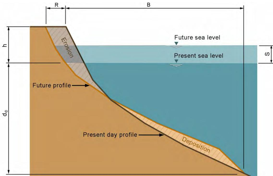
**Figure D3: Illustration of variables in the Bruun Rule**
