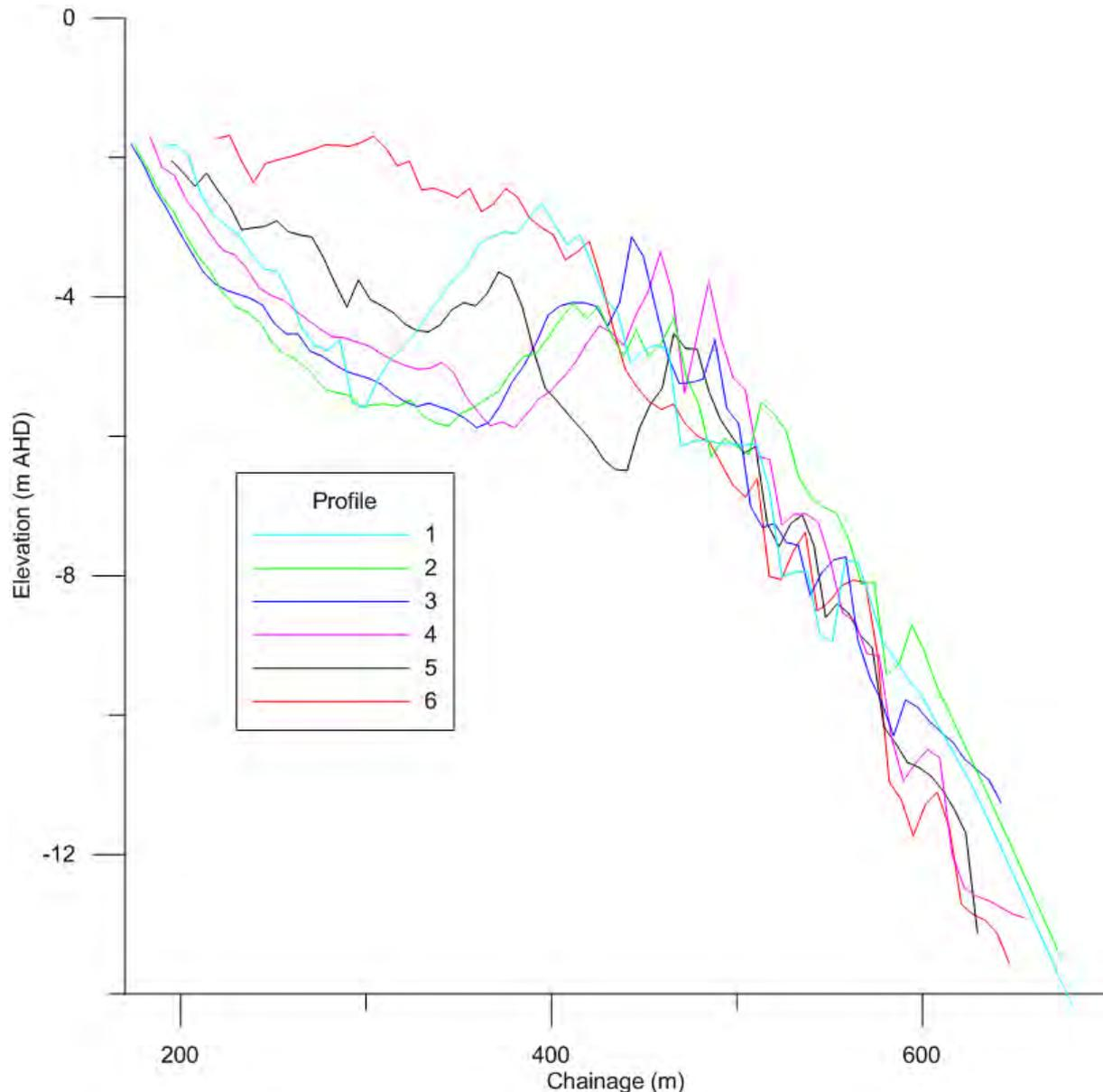
**Figure D5: Plots of chainage versus elevation for 6 profiles in Figure D4 (zero at western end of profile lines)**
