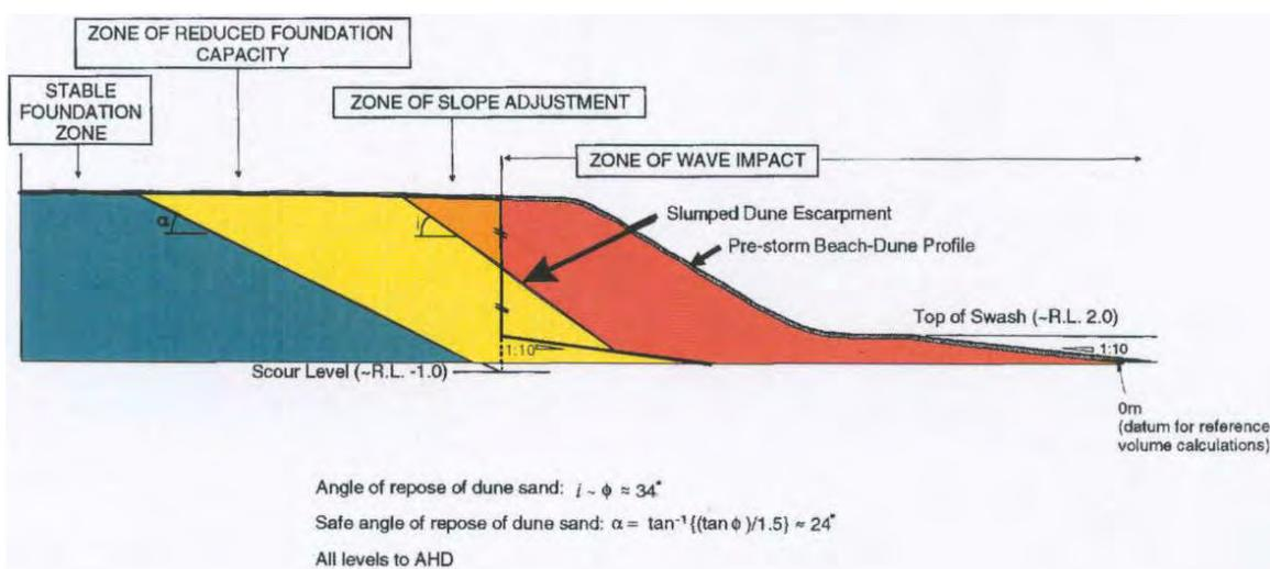
**Figure D2: Schematic representation of coastline hazard zones (after Nielsen et al , 1992)**
