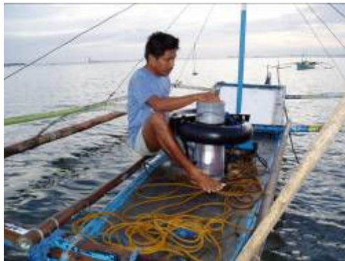
Photo showing CARE light being prepared for submersion
