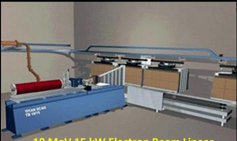
**10 MeV 15 kW Electron Beam Linear** Accelerator and Process Conveyor. Shielding removed to view the overhead power and conveyor system
