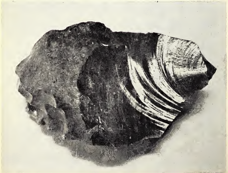
Obsidian, showing conchoidal fracture and sharp edges.
