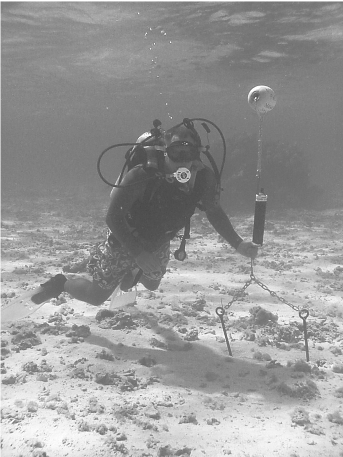
Figure 4. Diver with a VR1 autonomous acoustic receiver anchored to the seafloor with sand screws.
