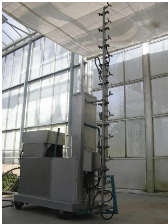
Figure 9. The robotic sprayer used to apply the spray
