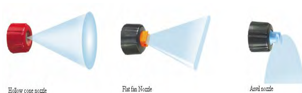
Fig. 5.3 Types of spray pattern produced by a hollow cone, a flat fan and an anvil nozzle.
