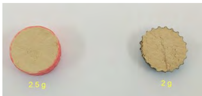
Fig. 5.8 Measuring pesticides (powders): 2.5 g (Coca-Cola bottle top (left); 2 g beer bottle top (right)
