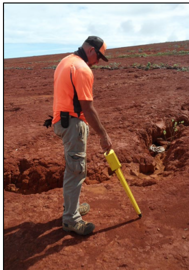
Figure 55 EOD Technician and Schonstedt metal detector on Kaho'olawe
