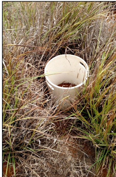
Figure 56 An 8" diameter infiltrometer
