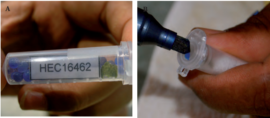
● Fig. 66. Silicagel-dried specimens. A., Eppendorf with silicagel, seaweed fragment and label; B. Indicating that the eppendorf has been used.
