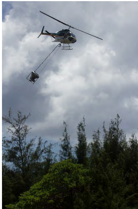
Figure 3. Helicopter rodenticide application using a bait hopper.
