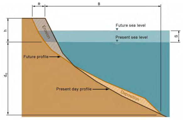
Figure D3: Illustration of variables in the Bruun Rule
