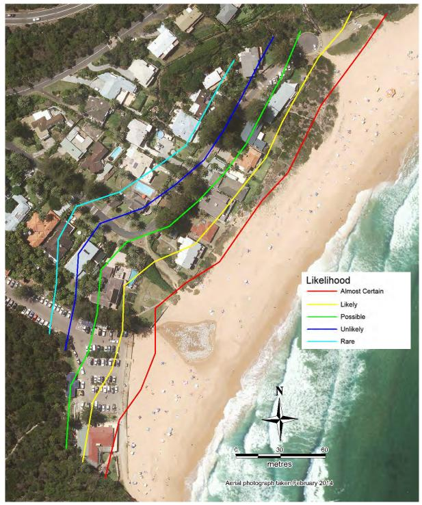
Figure D7: Likelihood lines at Bilgola Beach for Type 1 procedure (no recession included) for 60 year design life (to 2075)
