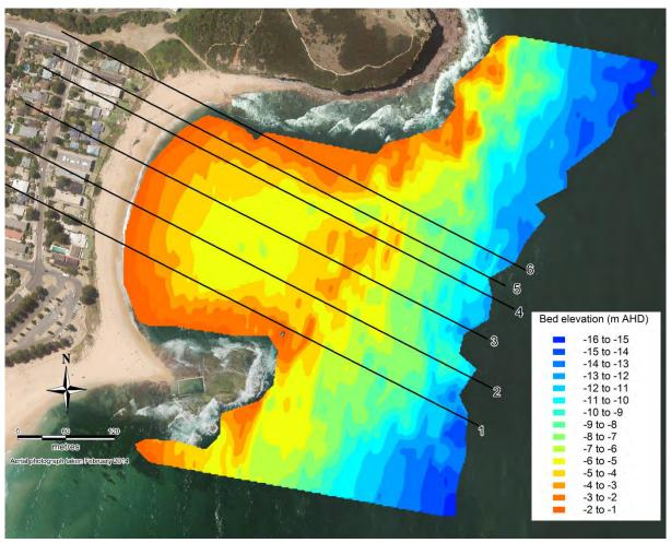
Figure D4: Bathymetric contours (relative to AHD) at Basin Beach from May 2014 OEH survey (1m contour interval)
