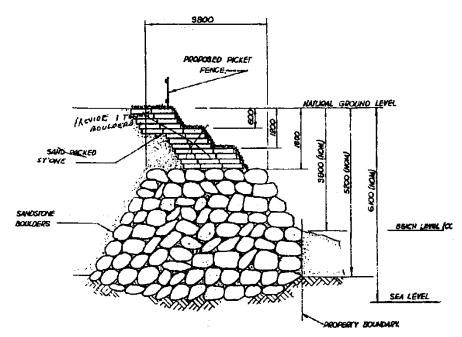
Figure A25: 1978 design drawing for 23 Surfview Road revetment from WRL (1999), note upper section as drawn has hand written notes showing this was deleted and replaced by boulders
