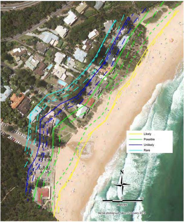
Figure D9: 95% (dash dot line), 50% (solid line)and 5% (dashed line) exceedance recession scenario likelihood lines at Bilgola Beach for Type 2 procedure for 60 year design life (at 2075)
