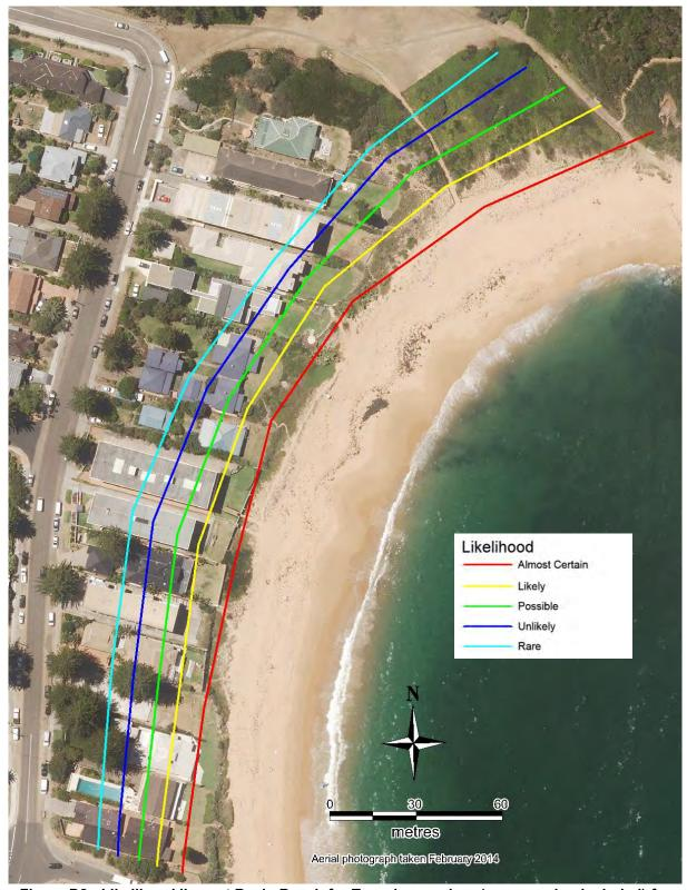
Figure D8: Likelihood lines at Basin Beach for Type 1 procedure (no recession included) for 60 year design life (to 2075)
