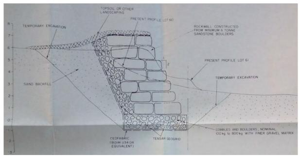
Figure A22: As-constructed drawing of seawall at 11 Surfview Road
