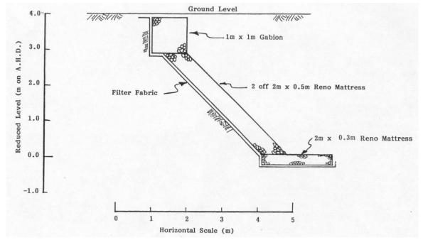
Figure A14: Typical cross section of gabion revetment at 21 Bilgola Avenue (from Patterson Britton & Partners, 2005)
