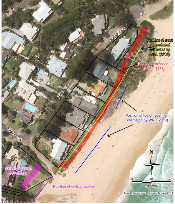
Figure A10: Extent of Allen Avenue rock revetment visible in 1978, estimated crest and toe position of rock revetment from WRL (2013), vertical seawall position seaward of 21 Bilgola Avenue, and location of gabion revetment at 21 Bilgola Avenue
