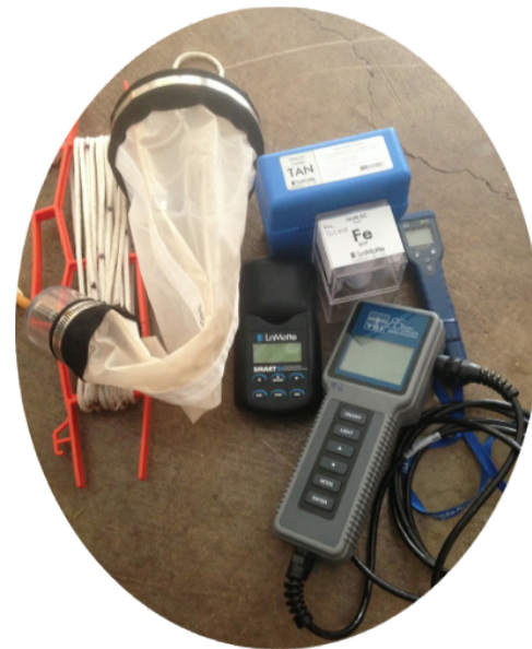
Above, from Left to Right: Tool used for plankton tow, LaMotte meter with Tannin & Iron reagents, pH meter, and YSI meter ( bottom ).
