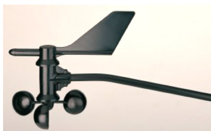
Figure 1.a. Anemometer used by MWS. There are two parts, a wind vane that measure direction and wind cups that measure velocity
