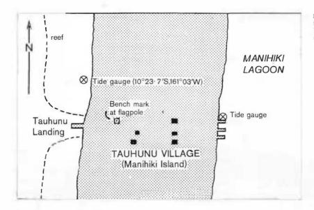
FIGURE 2: Sketch map showing the positions of the tide gauge in the ocean and lagoon, and the bench mark to which mean sea level is referred (see also the photograph, *figure 6*, p. 8).
