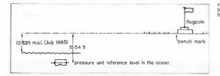
FIGURE 3: Diagram showing the mean sea level (m.s.l.) in the ocean, with reference to the bench mark
