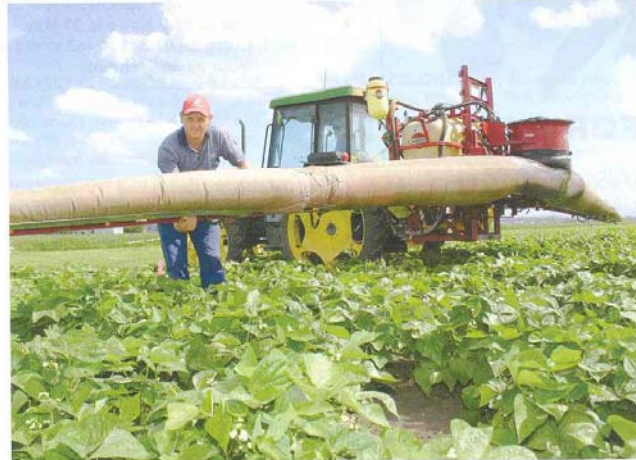
The air assisted spray rig used in the bean spraying trial at Gatton
