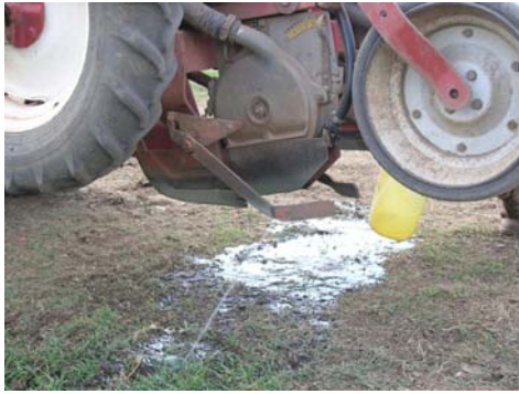
Photo 3. Soil application of imidacloprid showing position of injection line at rear of planting shoe.
