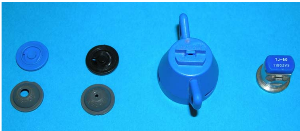
Figure 38. Nozzles used in trial. From left to right Hardi 1553-40 with blue swirl plate (fine hollow-cone), Hardi 1553-14 with black swirl plate (medium hollow-cone), Hardi ISO LD-110 03 (low-drift flat-fan)& Tee Jett TJ-110 03 (twin flat-fan).
