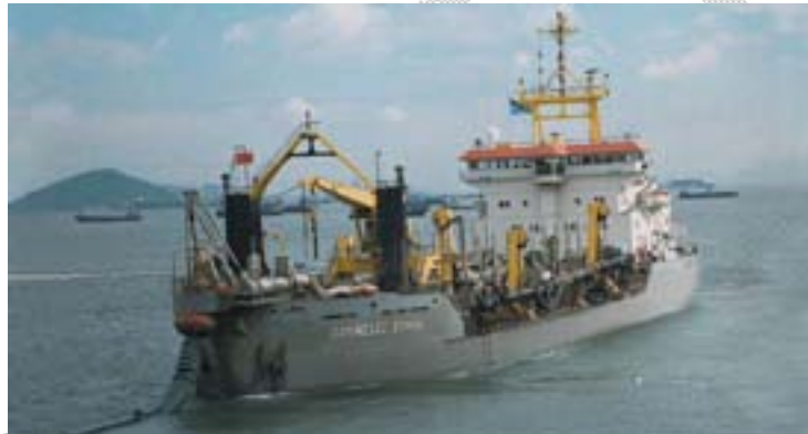
Figure 4-5: Example of Trailing Suction Hopper Dredge (TSHD)
