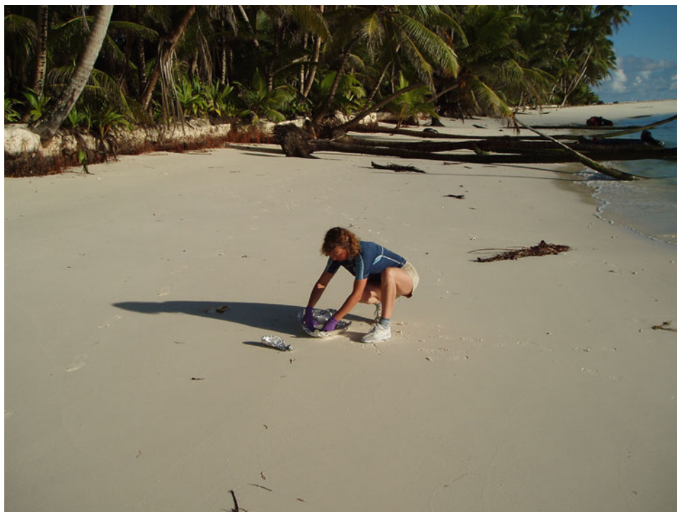
Fig. 21.1 Great Chagos Bank, eastern side of Eagle Island. Collecting sediment samples at low tide for subsequent analysis of PFOS and related compounds. The top approx 1 cm of sediment was removed and placed in dichloromethane pre-cleaned aluminium containers. Samples
