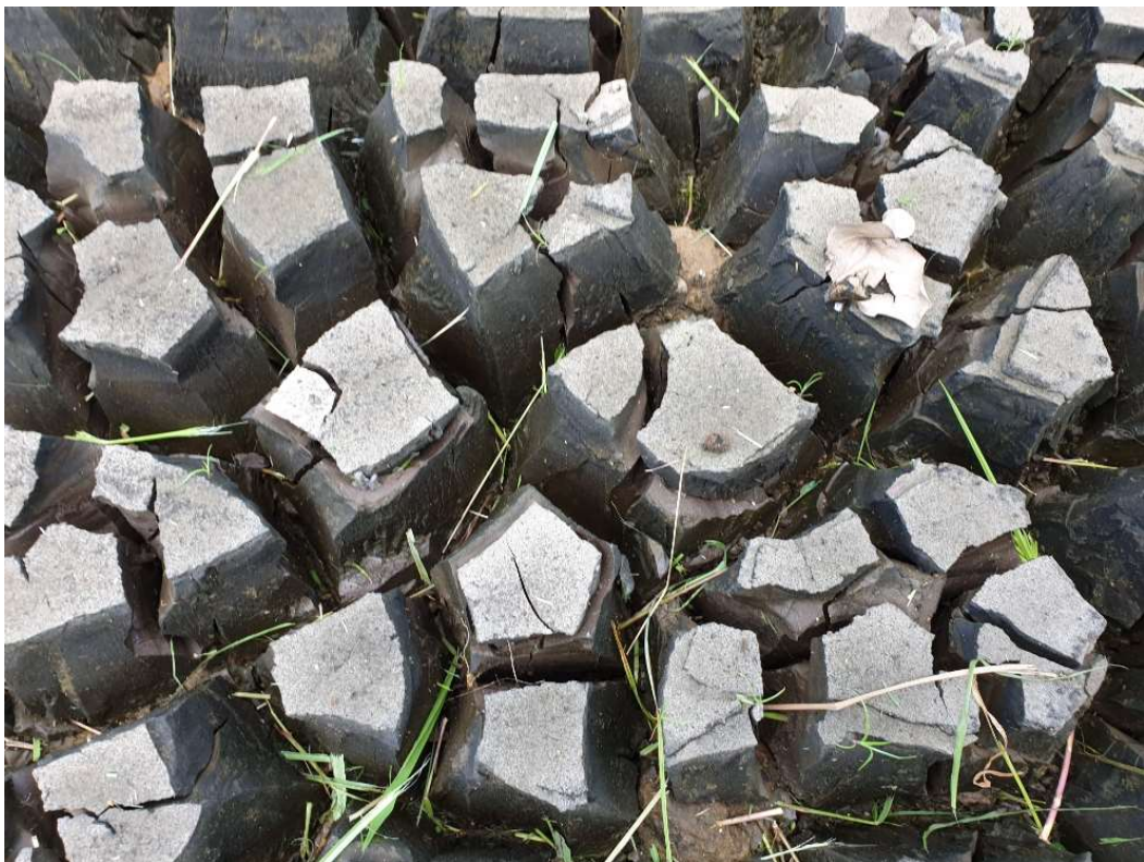
Figure 16 - Ngatoe scour pond(12 Jan 2021). Residuals are dry at the top and wetter at the bottom
