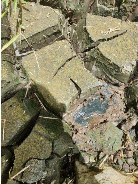
Figure 17 – Dried residuals in the Tupapa standby pond (Feb 2021, measured at 13-18% DS)
