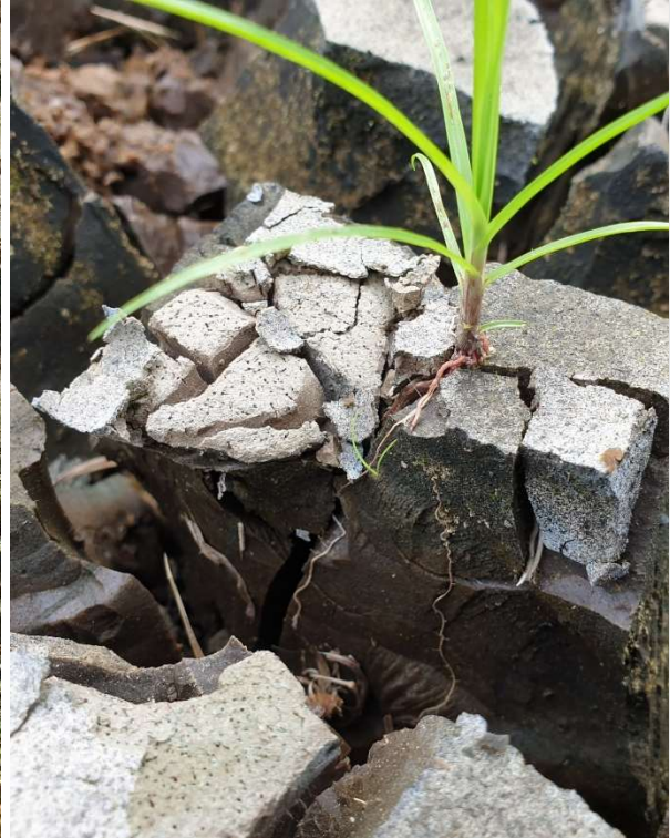
Figure 18 – Dried residuals in the Ngatote scour pond (25 Jan 2021, measured at 18% DS)
