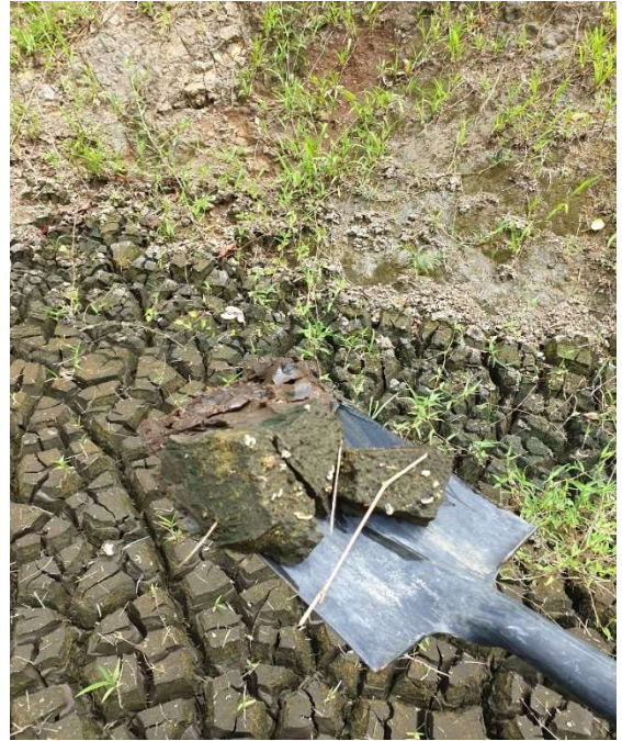
Figure 22 – Spade test at Tupapa (approx. 13-18% DS)
